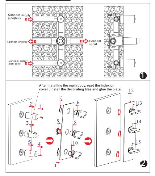
Read the Installation Fig and confirm the installing position.
