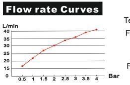
Test pressure: 1.6MPa (16bar) Flow pressure: Min 0.05MPa Max 1.60MPa Recommended pressure:
