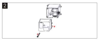
(2)Loose the M5 screw in the control box and open it.
