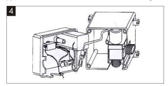
(4)Connect the plug of power supply and the one of valve together, close the box and fasten with M5 screw.
