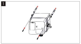
(1)Fasten the control box on the wall over 50cm of the floor with the screw.
