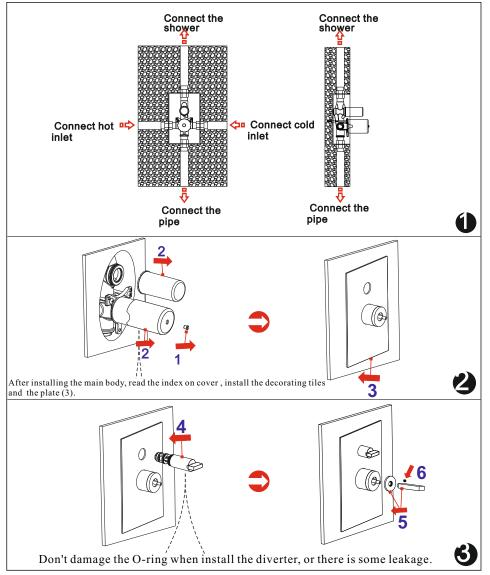
Attention: the inner radii of the G1/2 connection pipe is not less than  $\phi$ 13mm.
