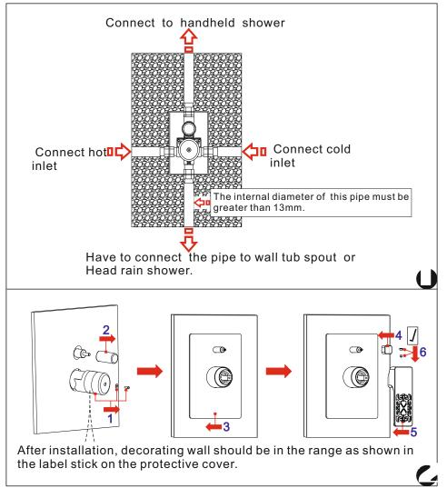
**\*** Read the Installation Fig and confirm the installing position.
