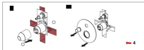
After installing the main body, read the index on cover , install the decorating tiles and glue the plate (4).
